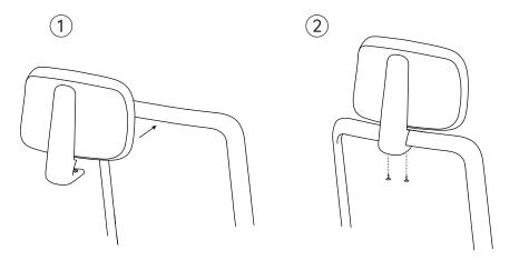
Attach **Headrest** to the top rear of the chair back frame. Align the holes on the **Headrest** base to the chair frame, insert both **Headrest Screws** (x2), and tighten with the **Hex Allen Key**.
