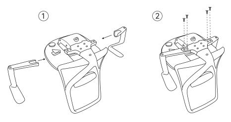
While the seat is still up-side down, insert the **Armrests** (x2) into both sides of the **Bridge**. Next, attach with the **Armrest Screws** (x4), and tighten with the **Allen Key**.
