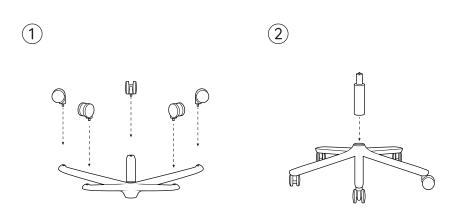
With the **Star Base** upside-down, push the **Casters** (x5) into each hole with a fair amount of force (they should 'pop' in). Once completed, turn over so the casters on are on the floor and insert the **Cylinder** into the **Star Base** with the larger end on the bottom.
