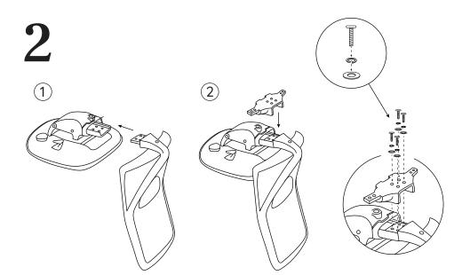
With the **Seat** upside-down (either on your lap or on top of the shipping box), align the **Backrest** mounting bracket onto the seat as shown. Place the **Bridge** over the mounting bracket and attach with the **Backrest Screws** (x4), **Lockwashers** (x4), and **Washers** (x4). Screw tight with the **Allen Key**.
