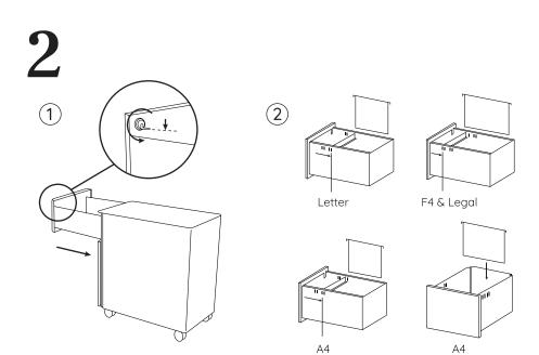
Before closing the drawer, turn the key so the bolt lock is facing down. Install the File/Folder Hanger (x1) in whichever orientation works best for you.
