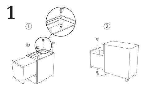
Place the filing cabinet upside down on a flat and clean surface. Open the bottom drawer, install the Locking Casters (x2) at the front of the cabinet, and the Non-Locking Casters (x2) at the back. Secure the Casters with the Lock Washers (x4) and Nuts (x4) using the included Wrench. Mount the balancing wheel to the underside of the bottom drawer with the Snap Pin (x1) from inside the drawer, ensuring the balancing wheel is curved towards the drawers.
