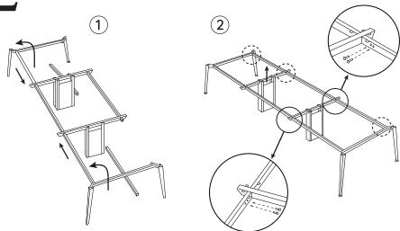
Starting at one side of the frame, carefully flip the first leg assembly right-side up and connect the frame. Repeat on the other side of the frame. Install the remaining Side Rails (x2) and screw all joints together with the Frame Screws (x2 per joint).
