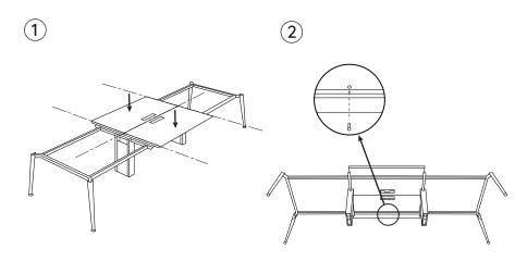
Align and center two Desk Tops (x2) in the middle of the assembled frame. From below, attach the desktops to the frame with the Desktop Screws (x12).
