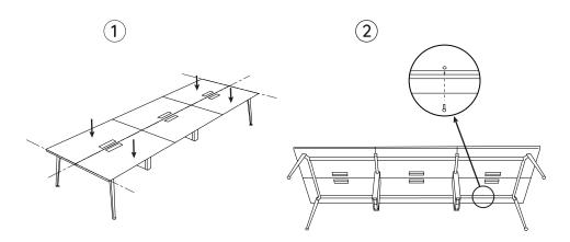
Align and place the remaining Desk Tops on both sides of the assembled frame. From below, atach the desktops to the frame with the Desktop Screws (x24).
